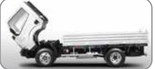
Tiltable Cabin in Any Gear – Ease of Serviceability
